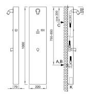
0,1 ? 1,0 MPa 12V, 50Hz 6VA ZAC 1/20 (max. 3 x BSZA) ZAC 1/50 (max. 8 x BSZA) ZT 1 10 sec. ? 42,5 min.  $2\ x$  of the preconfigured period of the water flow 12 kg
